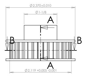
**NOTE: CORED PULLEYS** HAVE 1/16" THICK RIBS, REINFORCEMENT
